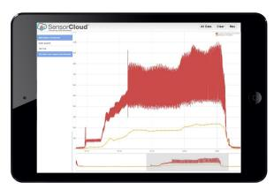
Live performance monitoring - With SensorCloud monitoring, equipment performance can be tracked during operation for failure conditions. Data can be analyzed further for predictive modeling.
