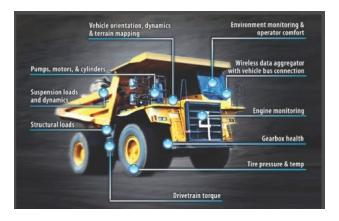
Large machinery in a high vibration environment -Measuring machine structural and component fatigue is necessary to prevent breakdowns and improve design.
