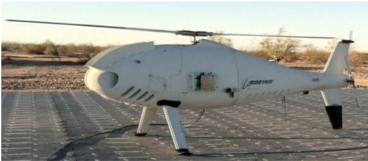
**Multiple technology requirements** - Flight testing of the UAV included collecting in-flight data from torque, strain, vibration, and temperature sensors, and a GPS-integrated inertial measurement unit.
